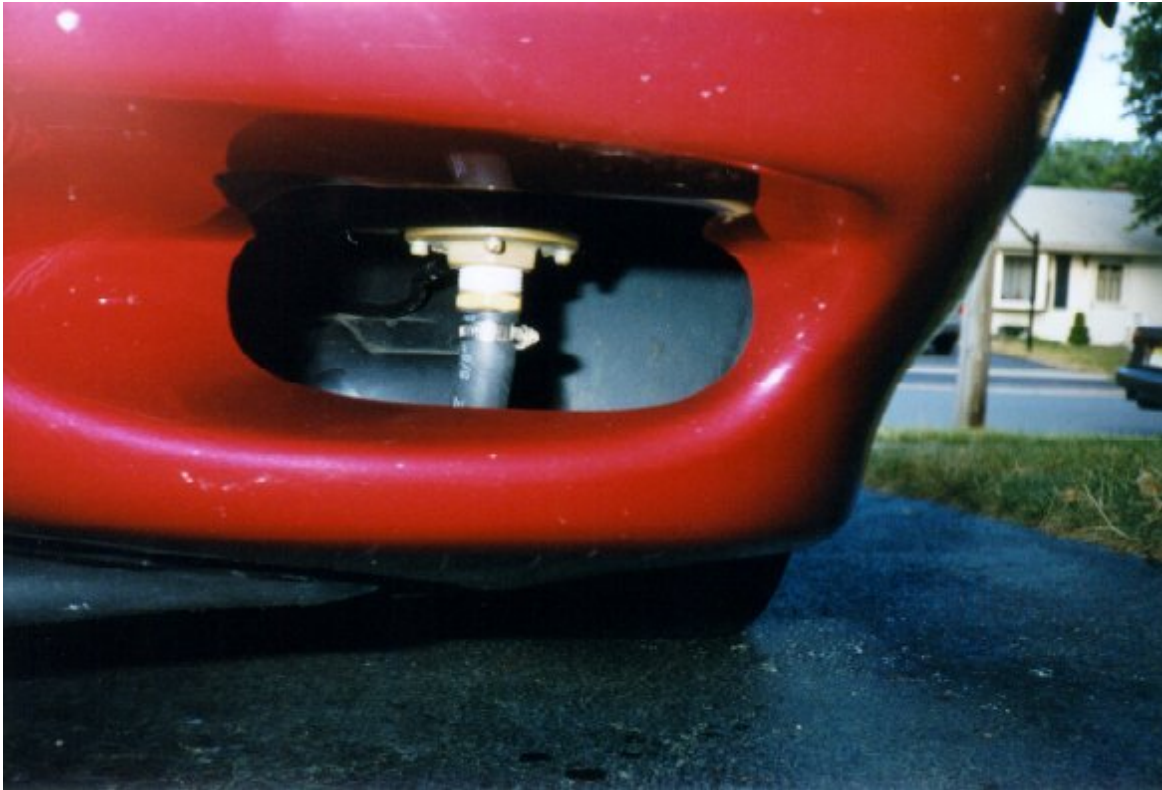
Water pump mount location viewed through the fog light hole
