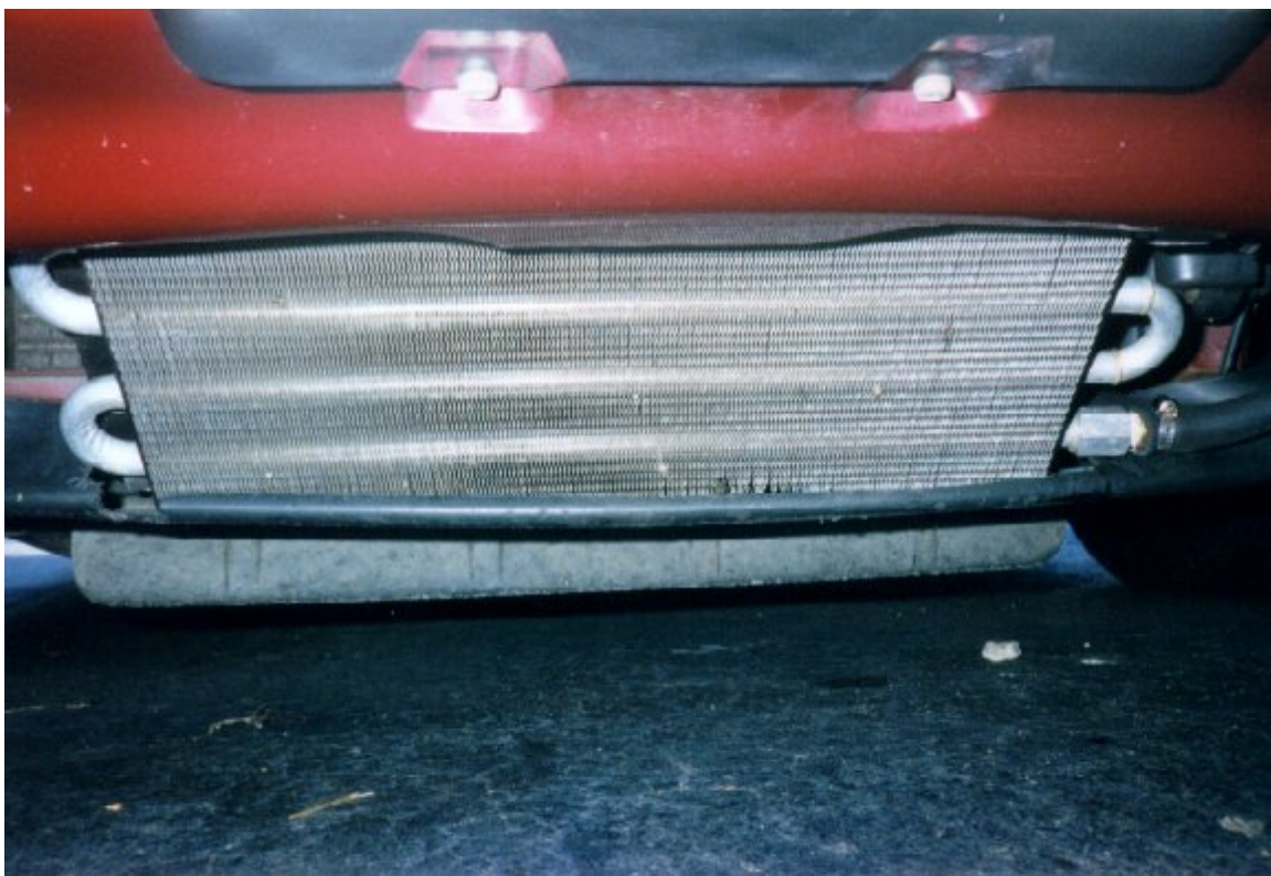
Heat exchanger mounting on '94 - '95 cars
