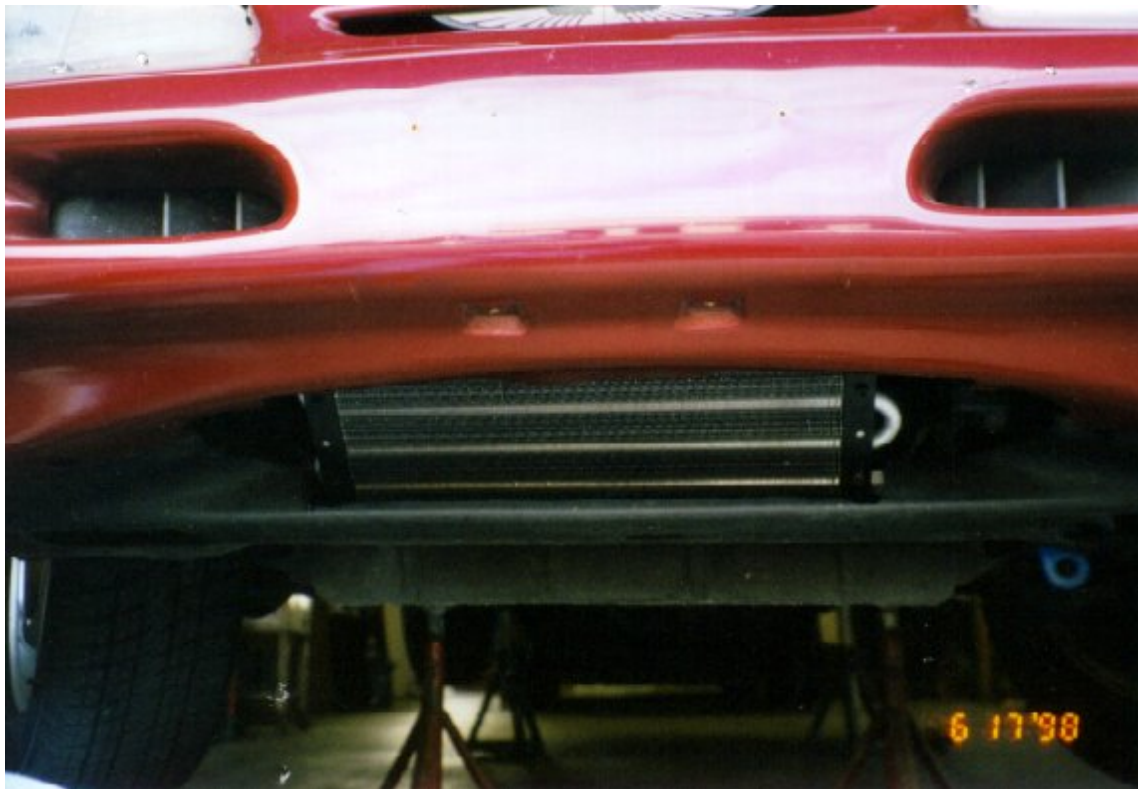
Cut support tab off from under license plate bracket
